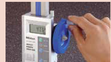
Large, smooth slider-feed wheel
